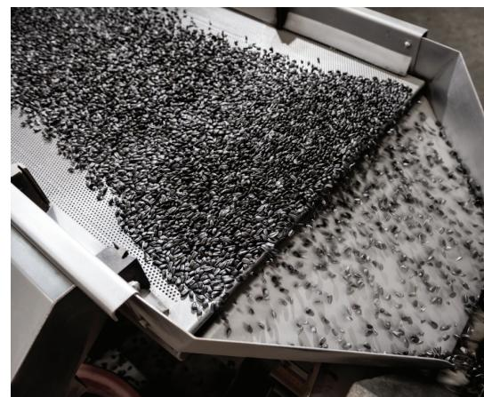
The fluid bed dryer is used for the processing and refining of waste products for their reuse, e.g. in the production of animal feed or the processing of grain sludge from breweries. Another use is for drying coarse minerals such as sand and gravel. Our engineers have developed fluidized bed dryers to ensure optimal results while minimizing abrasion. The unique drive allows us to create a fluidized bed as large as the product requires.
