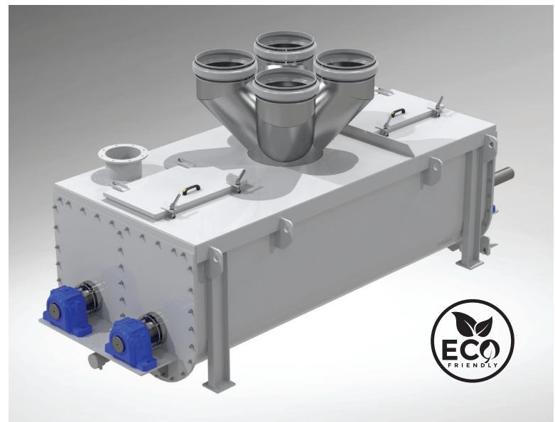
Plow or shovel-type paddle tools rotate in a special arrangement on the mixer shaft in a horizontal, cylindrical drum. The result is swirling of the mixture, which constantly draws all the product particles into the mixing process. The creation of dead spots or slow movement in the mixing drum is avoided, ensuring thorough mixing of raw materials. In some cases, separately driven high-speed knives can be installed to achieve the required mixing effect.
